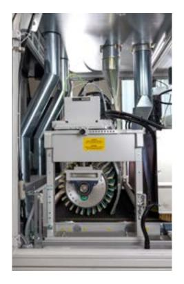
Heesemann sanding machines can be equipped with an extensive range of brush units featuring different heads for sanding and structuring. The brush units can be positioned at an angle to the feed or can oscillate.
