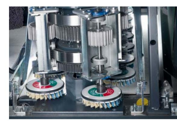
The RUT disc brush unit consists of 18 disc brushes arranged to enable unmatched quality when sanding contours. All of the areas are sanded evenly in different directions.
