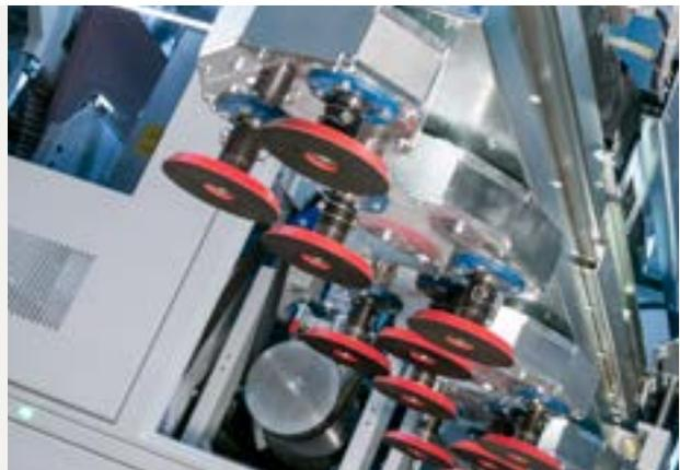
For easy mold or application changes, the DB-S can be pulled out of the side of the machine on integrated rails. All platens are thus freely accessible. Thanks to **quick-release fasteners**, this can be done within a few minutes.
