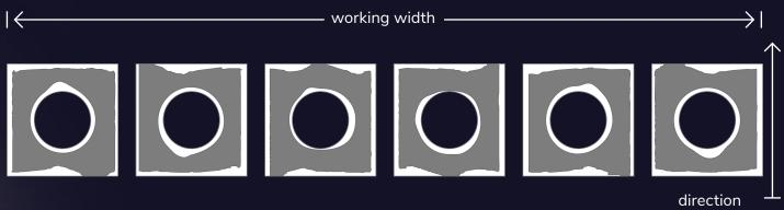
Uneven rounding results influenced by the position and direction as well as low feed rates. The illustration clearly shows the non-uniformity generated by this process.
