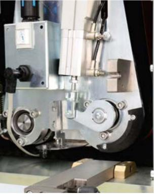
**Head locking**Safe and simple quick-lock heads to rapidly change the sanding belt
